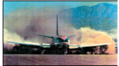
Untreated runways can lose 2" of material per year requiring hundreds of thousands of dollars to replace.
